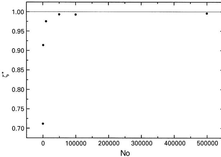
Fig. 4. Branching ratio for different system sizes ( $\rho = 2$ ) for the global load sharing case. As the size of the system is increased the value of the branching ratio for the last non-catastrophic avalanche approaches unity.
