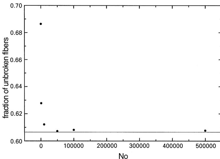
Fig. 5. Fraction of unbroken fibers just before the final breakdown in the probabilistic model of the global load sharing case as a function of the system size ( $\rho = 2$ ). The horizontal line shows the exact value in the thermodynamic limit.
