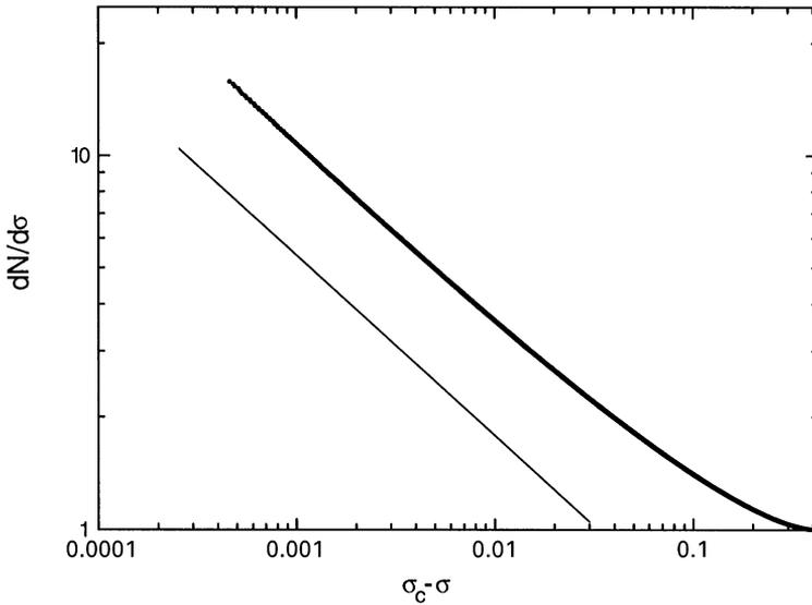
Fig. 1. Rate of fiber failure as a function of the distance to the critical point for the continuous version of the probabilistic global load sharing model for a system of  $N_0 = 50\,000$  elements and  $\rho = 2$ . A line with the mean-field value  $\gamma = \frac{1}{2}$  of the exponent is plotted for reference.
