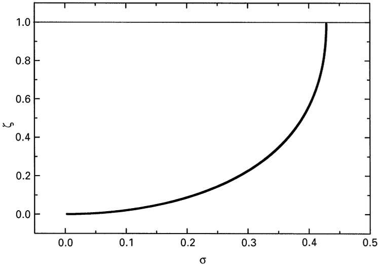
Fig. 2. Evolution of the branching ratio as the critical point is approached in the continuous probabilistic method ( $N_0 = 50\,000$ ). Note that at the critical point the branching ratio reaches the unity.
