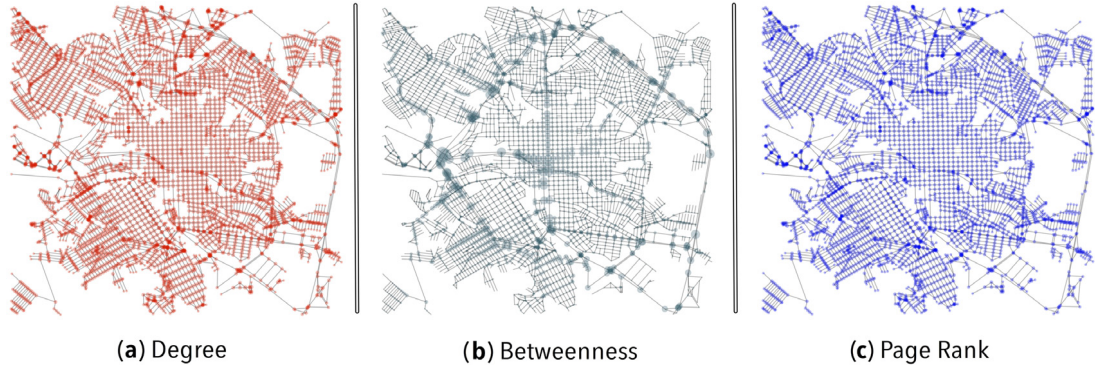
Fig. 3. Comparison of three different centrality measures: degree in (a), betweenness centrality in (b) and Page Rank in (c). The size of the nodes are proportional to the centrality of the node. The network used is the São Carlos road map, extracted using the Python library OSMNX (Version: 0.5.1 – https://github.com/gboeing/osmnx ).
