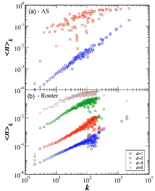
FIG. 4. Average number of covered vertices (servers)  $\langle n \rangle_k$  restricted to vertices with the same degree  $k$  for several values of  $d$ . The figures show that for disassortative graphs (a), the servers should have a large capacity to serve a finite fraction of the graph even for small to moderate values of  $d$ . On the contrary, for assortative graphs (b), the fraction of servers is a negligible fraction of  $N$  up to large values of  $d$ .
