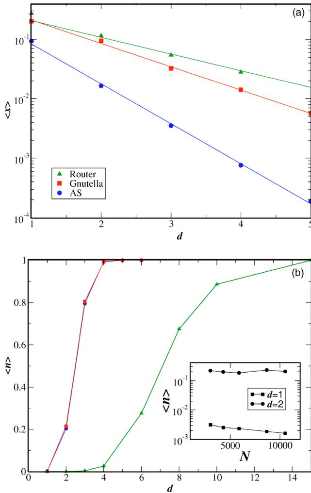
FIG. 3. (a) Average fraction of servers  $\langle x \rangle$  covering the graph for different values of  $d$ . The continuous lines are the best fits to an exponential decay. (b) Average fraction of vertices  $\langle n \rangle$  served by a server for different values of  $d$ . The inset shows the graph size dependence of  $\langle n \rangle$  for the AS graph and  $d=1, 2$ .
